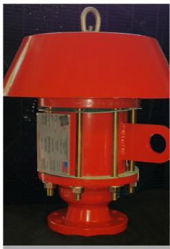
*The Paradox End of Line Flame Arrestors*, are designed for free venting while simultaneously preventing flame propagation of confined and unconfined low pressure deflagrations. They prevent an ignited atmospheric vapor cloud from propagating beyond the Flame Arrestor into the line or tank.
